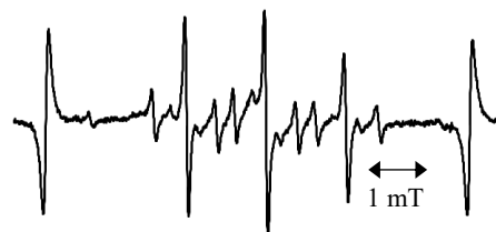
Fig. 2. ESR spectrum of PTT/MNP 1.0 wt% at 130 °C.
