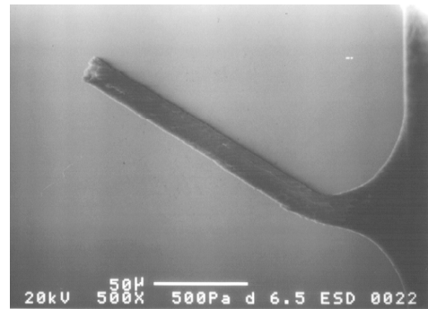
Fig.8 Electrode with diameter of 18\mu\text{m} and bending angle of 32^\circ for method B
